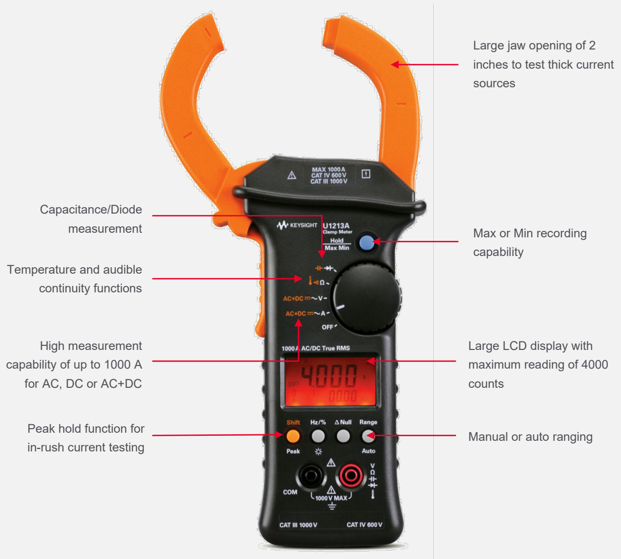
Figure 4. Front view of U1213A handheld clamp meter
